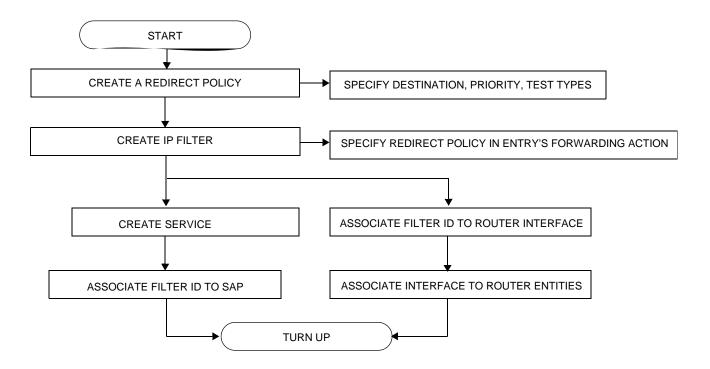
Figure 20: Filter Creation and Implementation Flow
